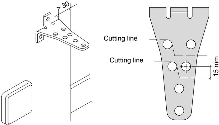
In order to properly cut the bracket start 15 mm from the hole center, as shown in the picture.
